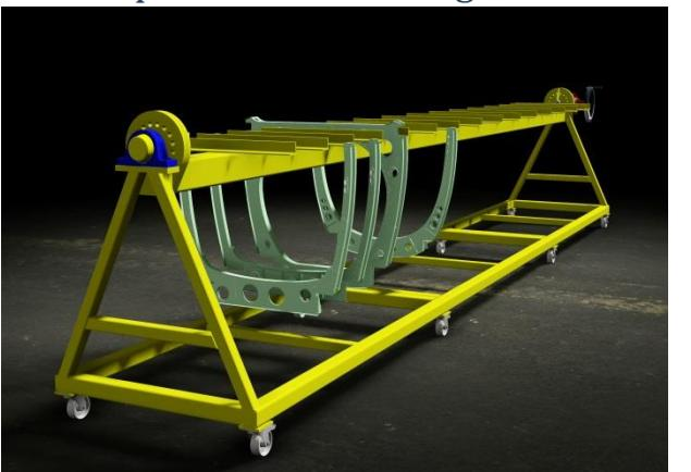
will be able to place each frame in its exact position relative to the fuselage datum line, and this will very quickly take on the line of this beautiful fighter. This will just be a temporary measure though, as the entire assembly is far too large to be accommodated within the Art Department permanently. However, it will be a huge leap forward for the project, and with our current efforts to secure funding for the Spitfire Education Centre, may
