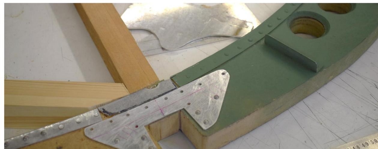
longerons and seat support, (see image above)...there are a total of 16! They are not particularly complicated, but with limited tooling take us a long time to make; however, we have now begun fitting some... Zoe has already made all of the intercostal brackets, so Frame 11 should be fully assembled and in final paint shortly.
