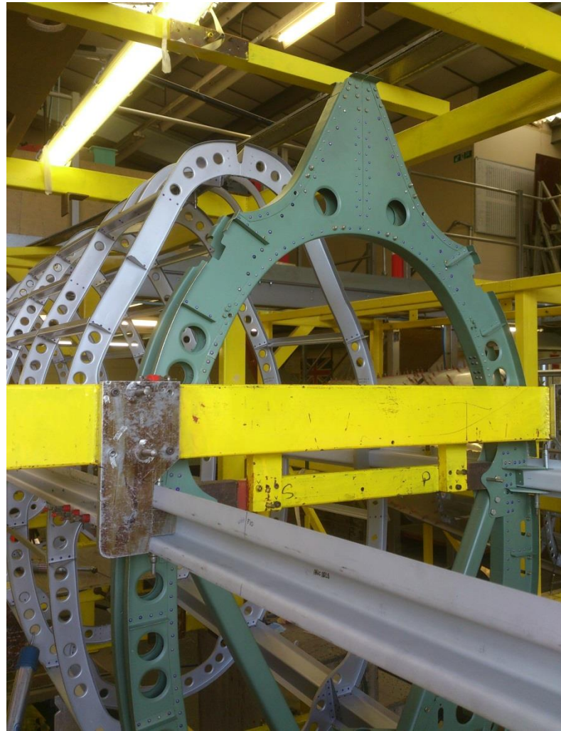
A MkV fuselage coming together in a jig
